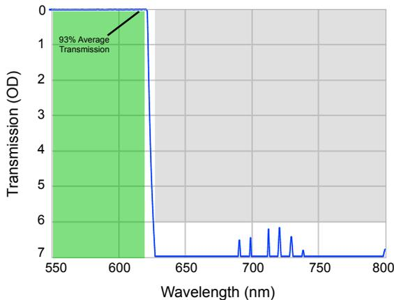
Figure 4: VersaChrome short-wave pass tunable edge filters maintain high transmission and deep blocking, even at AOI = 60°.
