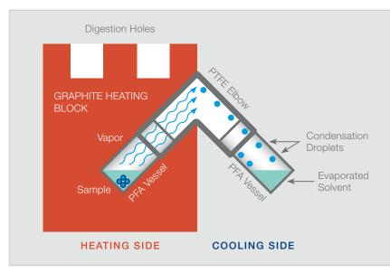
Evaporation of the reagent for separation or purification is made at constant, homogeneous and controlled temperature.
