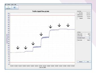
The realtime flow display enables you to optimise the pressure on the peristaltic pump tubing. The clamp was tightened by a half turn at each arrow.
