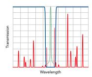
Versatile laser-blocking notch filter for both Stokes and Anti-Stokes measurements
