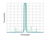
Laser-transmitting filter for both Stokes and Anti-Stokes measurements
